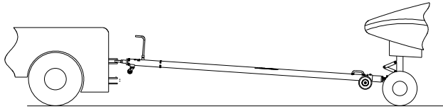
Incorrect Excessive Towbar Angle
