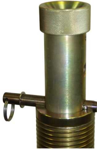
Ball Lock In Ram Protection Ring
