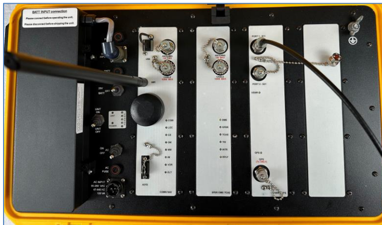
VSWR Setup with connection to Port 1
