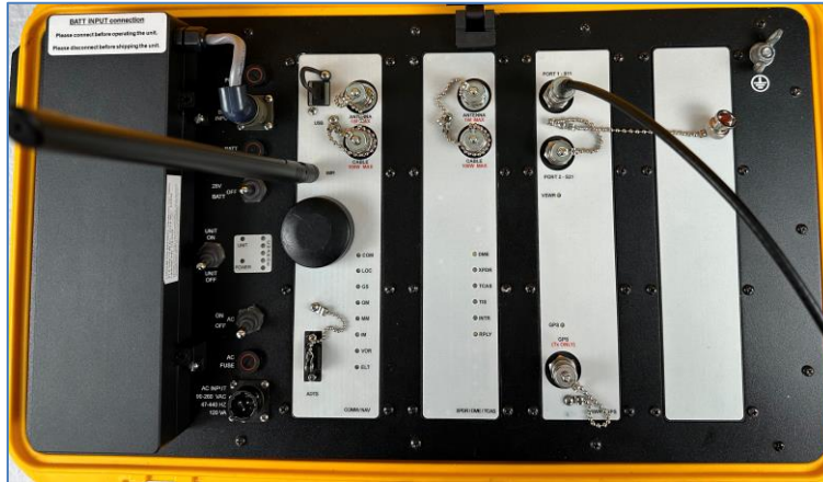
VSWR Setup with connection to Port 1
