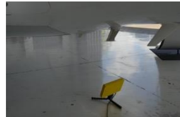
Good line of sight between Aircraft Antenna under test and ARTS 7000 test antenna.
