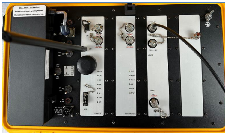
VSWR Setup with connection to Port 1
