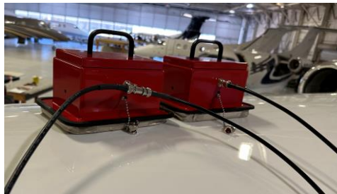
ARTS 7000 GPS couplers covering dual aircraft antennae.
