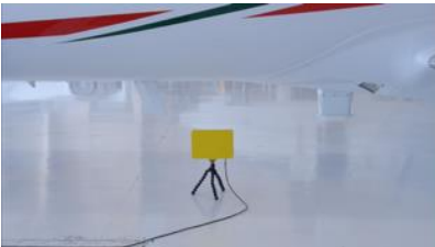
Good line of sight between Aircraft Antenna under test and ARTS 7000 test antenna.
