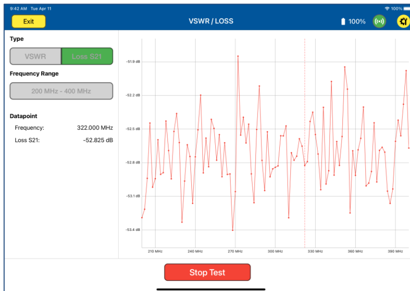
S21 Loss measurement.
