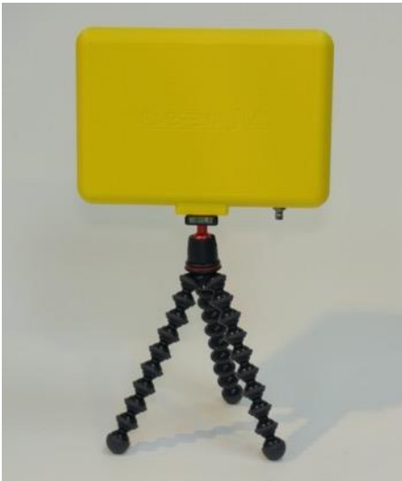
1. Pulse Antenna mounted on tripod.
