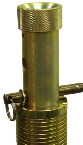
Washer On Top Of Ram Protection Ring
