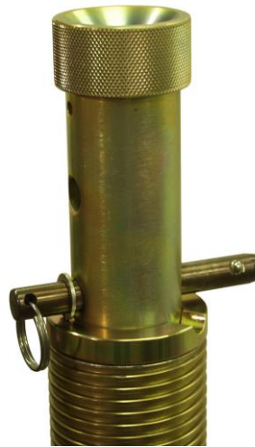
Washer On Top Of Ram Protection Ring
